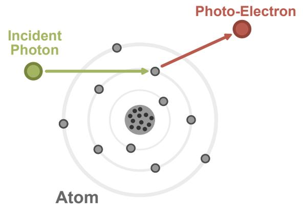
(b) Diagram of Photoelectric Absorption.
