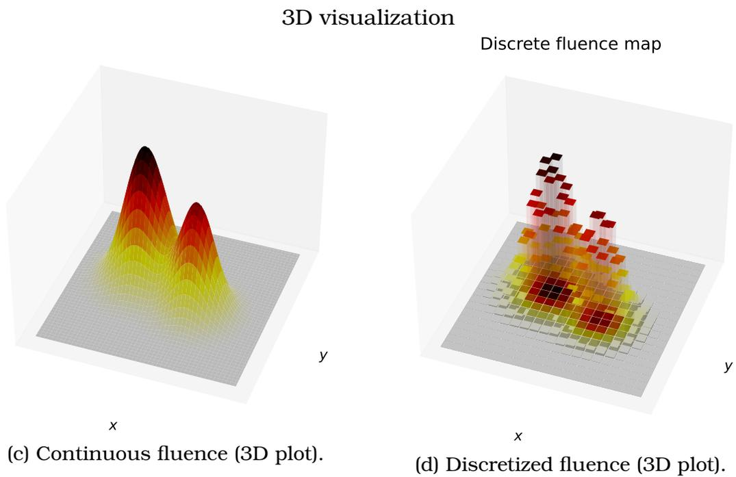
Figure 3.1: Example of a fluence discretized to  $20 \times 20$  bixels.
