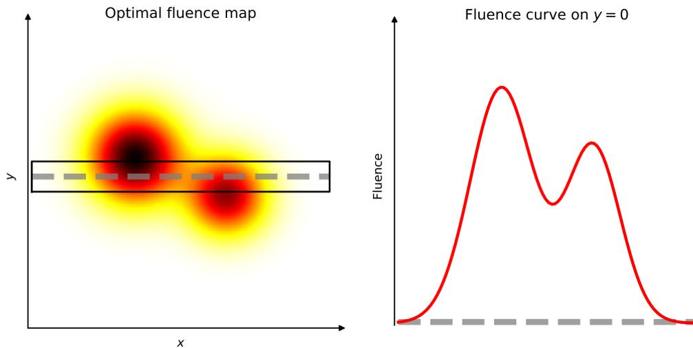
Figure 1.8: Example of a fluence map segmentation along a leaf pair axis.
