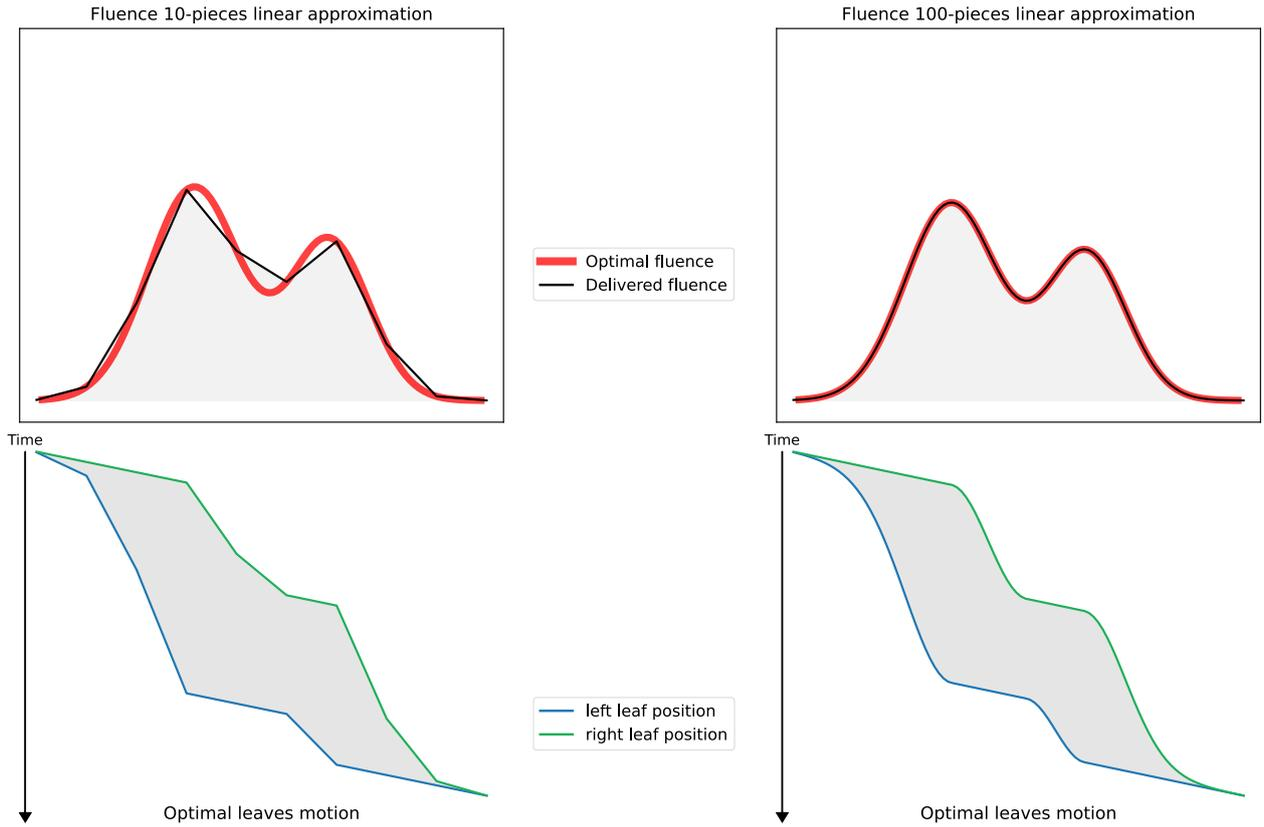
(a) Example of a fluence curve leaf sequencing, with the fluence approximated by a 10-pieces linear function.
